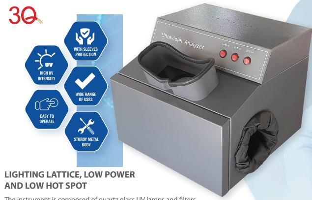
The instrument is composed of quartz glass UV lamps and filters, with wavelengths of the two sets of light sources; short-wave ultraviolet (254nm) and long-wave ultraviolet (365nm). The light source can be used for experiments after being filtered by a filter, and the two light sources can be used alone or mixed at the same time.
